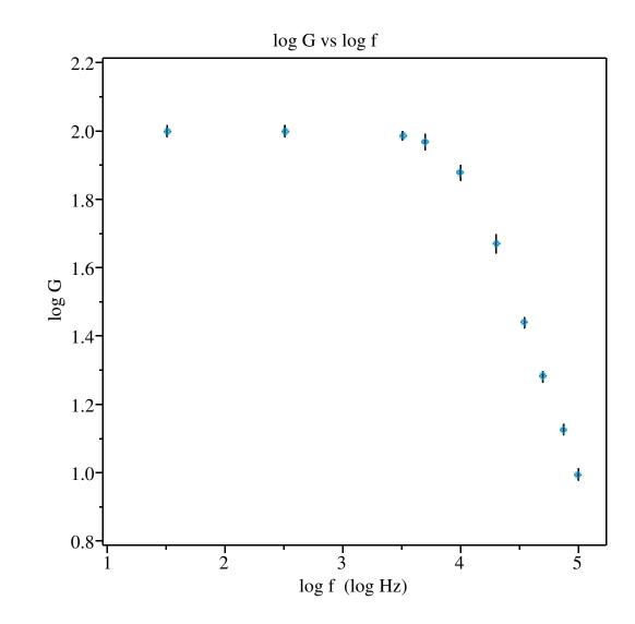
Notice that the slope of the high-frequency roll-off does not depend on whether we do a ln-ln plot or a log-log plot (as expected).
